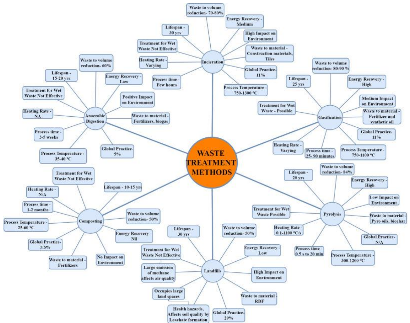
Figure 6. Comparative diagram of the technical features of various waste treatment methods. (Source: Sondh et al. 2024 https://doi.org/10.1016/j.scj.2023.101337 ).
